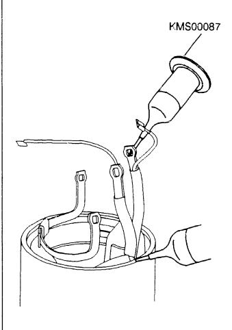
CHECKING AND REPAIRING COMPONENTS Checking excitation winding Use tester to check resistance values. Alternator tester: 0 684 201 200 (or Motortester) Resistance, shunt winding (24 V/5.4 kW): 960...1060 mOhm (24 V/6.6 kW): 750... 830 mOhm (12 V/3.5 kW): 240... 270 mOhm (12 V/3.6 kW): 220... 250 mOhm (12 V/4.0 kW): 160... 190 mOhm
